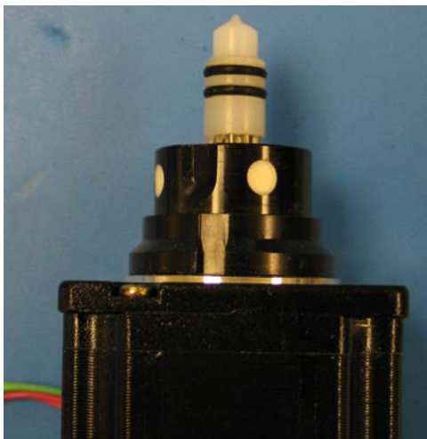
Figure 99: The High Pressure Valve Seal — Before Removal
