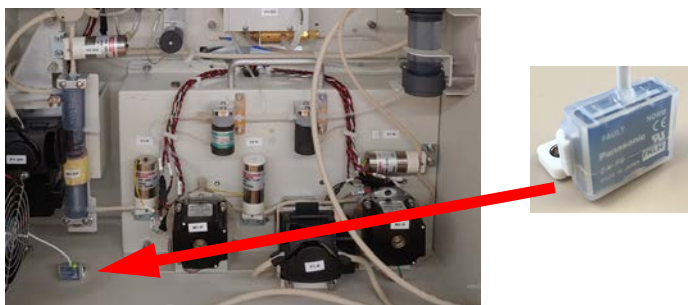
Figure 83: Liquid Sensor Location — Analyzer Enclosure
