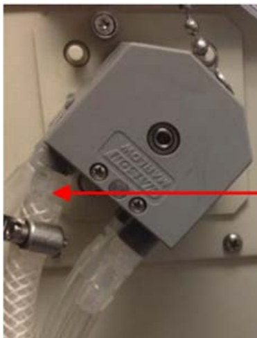
Figure 28: Overflow Mode — 2-Stream, External Sample Peristaltic Pump Position
