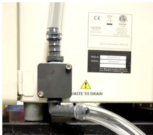
Figure 5: Connecting the Waste Lines on the Waste Block
