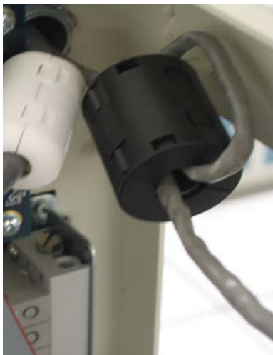
Figure 13: Ethernet Cable Passing through Ferrite
