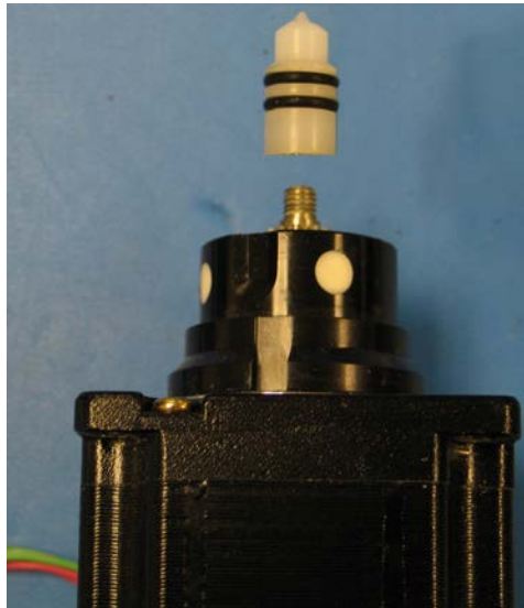
Figure 100: The High Pressure Valve Seal — After Removal
