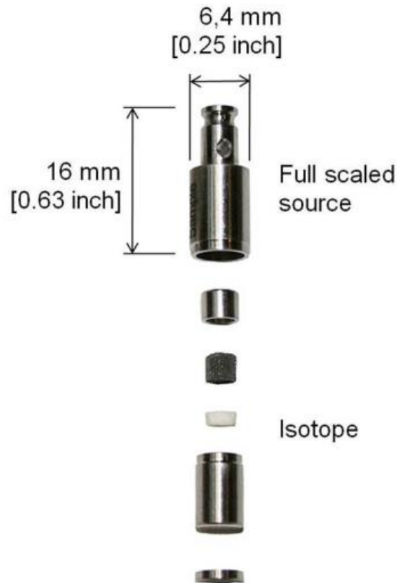
Picture: Cs-137 gamma source, model: VZ-79 Supplier: Eckert & Ziegler, Germany
