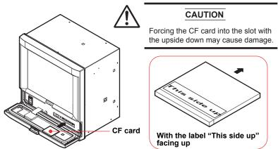
2. Insert the CF card into the slot.
