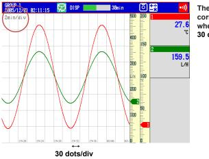
The sampling interval (the time corresponding to 1 dot) is 4 s when the trend interval is 2 min. 30 dots  $\times$  4 s = 2 min
