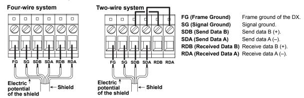
Recommended length of stripped wire: 9 mm. Recommended tightening torque: 0.4-0.5 N-m.
