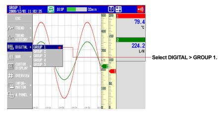
Press DISP/ENTER once to show the operation display of the selected group. To close the menu without switching the display, press ESC.
