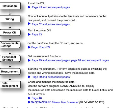
When using the DX for the first time, carry out the following procedure.
