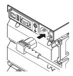
**3.** Check that the power outlet meets the conditions given in the table above and that the supply voltage is within the maximum rated voltage range of the power cord that comes with the package. Then, connect the other end of the power cord to the power outlet. The AC outlet must be of a three-prong type with a protective earth ground.
