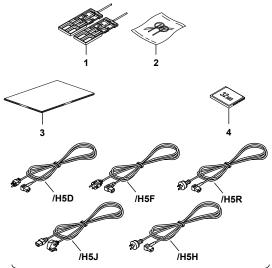
5. One of these power cord types is supplied according to the instrument's suffix code
