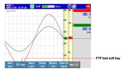
Press the Primary soft key once. The messages "FTP test is being executed" and "Execution is complete" are displayed. The test file (FTP\_TEST.TXT) is sent to the FTP server.
