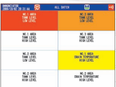
– Overview display – This screen lets you monitor the alarm status and numeric value for all channels.
