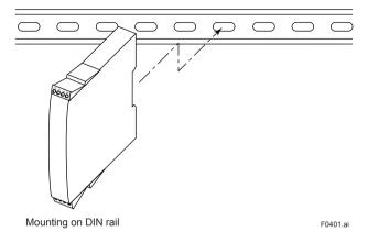
Figure 4.1 Mounting the Transmitter
