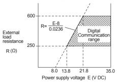
Figure 8.2 Relationship between Power Supply Voltage and External Load Resistance
