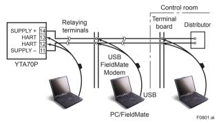
Figure 8.1 Connecting the HART configuration Tool
