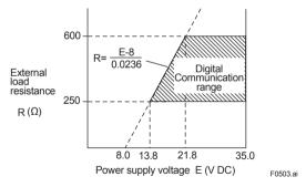
Figure 5.3 Relation between Power Supply Voltage and Load Resistance
