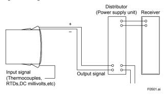
Figure 5.1 Loop Construction (for General-use Type)
