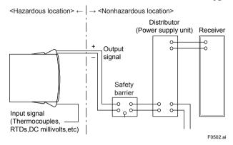
Figure 5.2 Loop Construction (for Intrinsically Safe Type)
