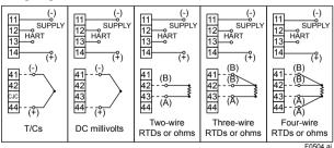
Figure 5.4 YTA70P Wiring Diagram
