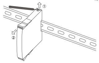
First, remember to turn off power supply and remove output signal cable. Detach the device from the DIN rail by lifting the lock.  $$_{\rm F0402.ai}$$
