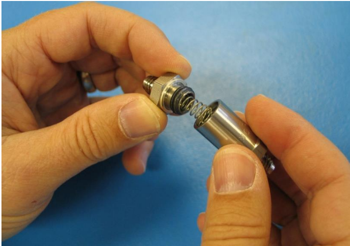
Figure 37: Opening the Filter
