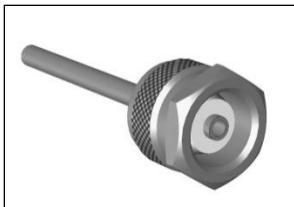
Figure 18: The Reducing Ferrule After Installation
