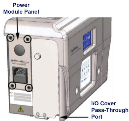
Figure 6: The Default Power Module Panel and I/O Cover
