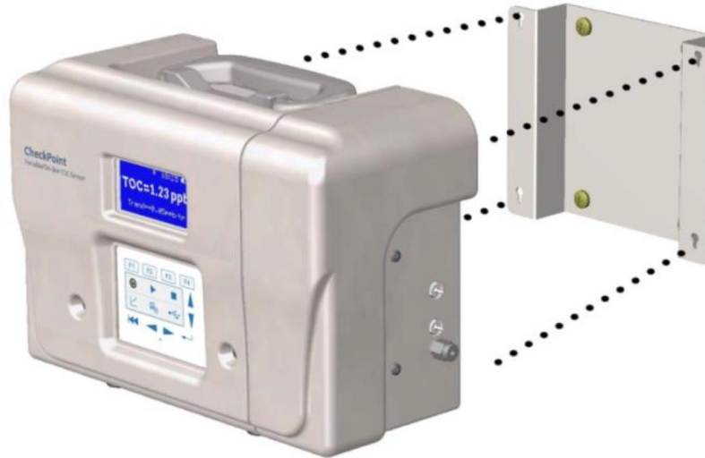
Figure 2: Mounting the Sensor on the Bracket
