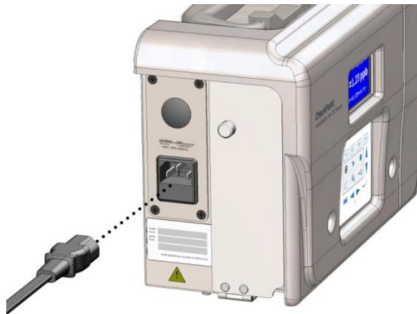
Figure 3: Installing the Power Cord
