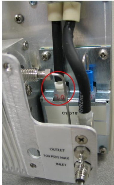
Figure 40: Removing the Sample Pump Inlet Tubing
