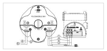
Connection of the battery and the solar panel
