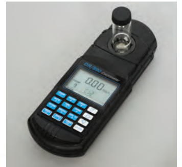
Measuring free available chlorine levels using a colorimeter: no chlorine detected in water after Atlantium UV treatment
