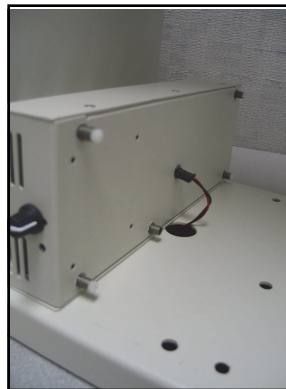
Figure 6: Connecting the Stirring Plate Wiring
