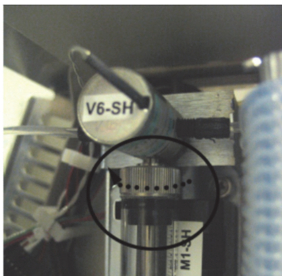
Figure 54: Unscrewing the Syringe Base
