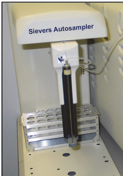
Figure 11: Lowering the Sievers Autosampler Arm
