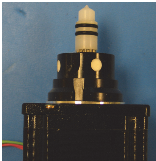
Figure 63: The High Pressure Valve Seal — Before Removal
