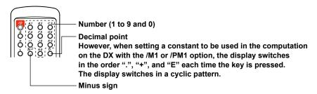
When a window for entering an equation is displayed on the DX with the /M1 math option, the character strings of computing elements are assigned to each key as shown in the following figure.
