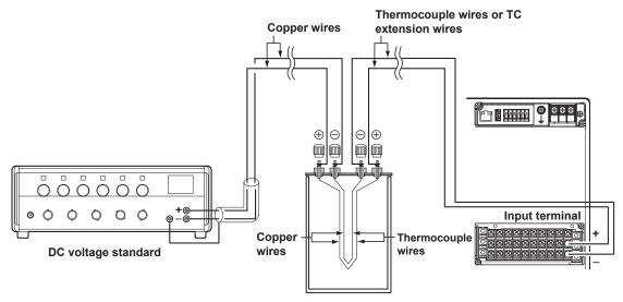
(0 °C standard temperature device ZC-114/ZA-10 by Coper Electronics)
