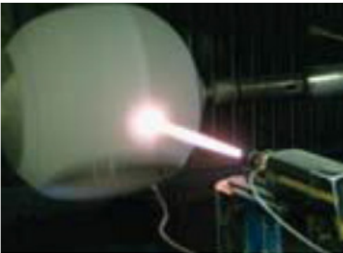
Figure 8 Hard coating done by HVOF technology
