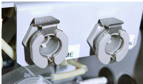
Figure 9: Metal Port Latches
