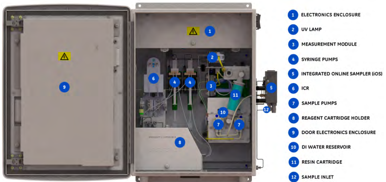
Figure 42: Interior Overview — Sievers M5310 C On-Line TOC Analyzer
