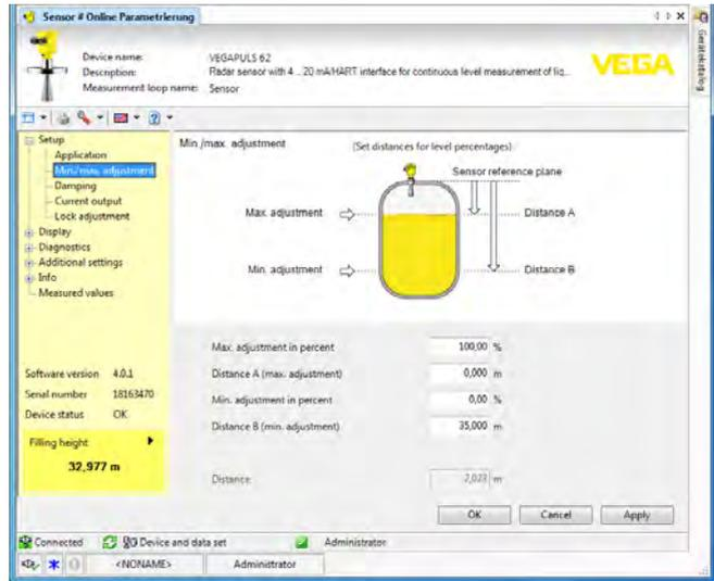
Fig. 10: DTM view VEGAPULS 62 online operation (synchronized)
