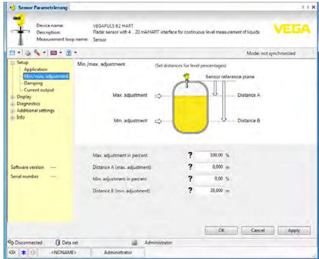
Fig. 12: DTM view VEGAPULS 62 offline operation (not synchronized)
