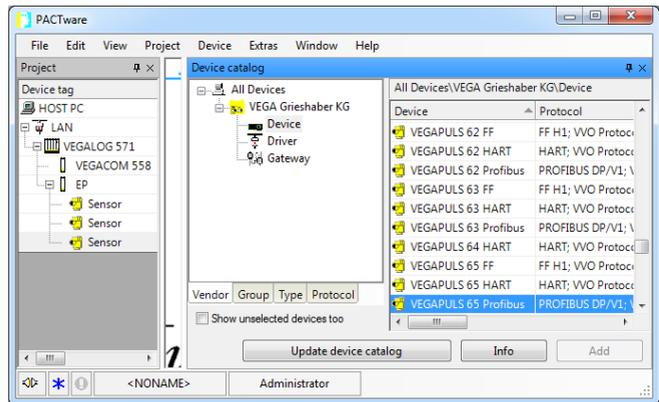
Fig. 8: Project VEGALOG 571 with Profibus PA sensors
