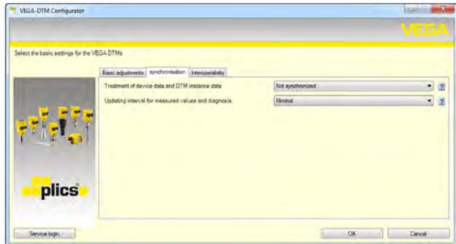
Fig. 11: DTM Configurator: Configuration of the data synchronization
