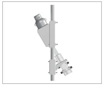
Fig. 15: 30° measurement setup on a pipeline with diameter 50  $\dots$  100 mm (1.97  $\dots$  3.94 in)
