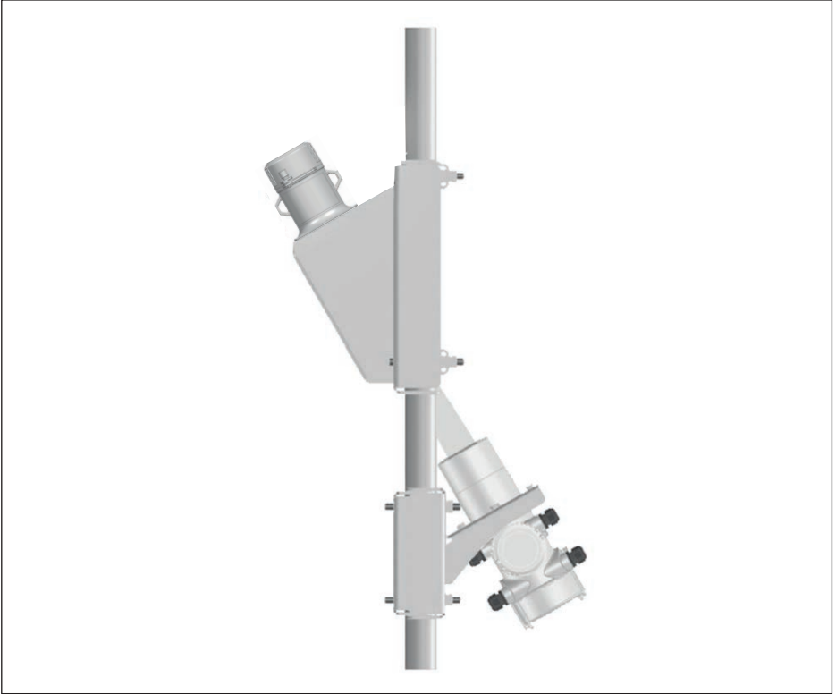
Fig. 45: Mounting brackets for diagonal mounting on pipes from 50 ... 220 mm (1.97 ... 8.66 in)
