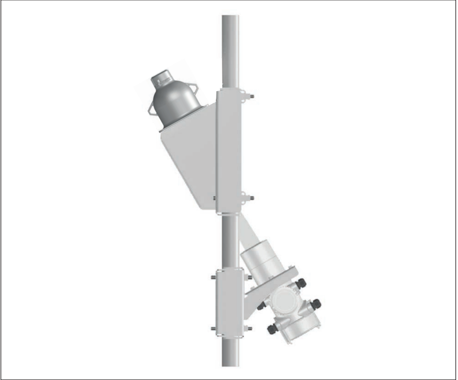
Fig. 45: Mounting brackets for diagonal mounting on pipes from 50 ... 100 mm (1.97 ... 3.94 in)
