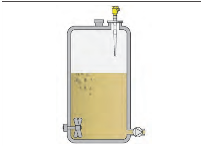
Fig. 30: Level measurement in a storage tank with VEGAPULS 65
