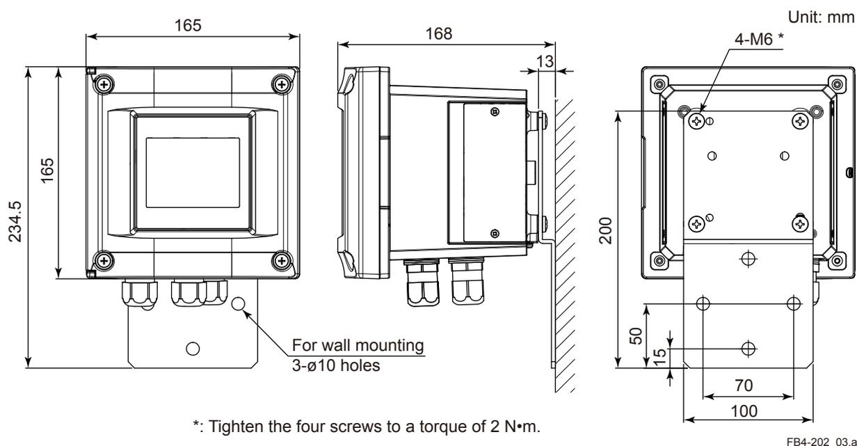
Note: The wall on which the analyzer is mounted should be strong enough to bear the weight of more than 8 kg.
