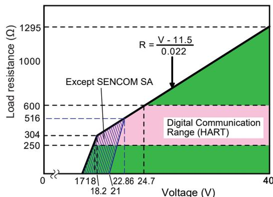
Figure 2 Supply Voltage and Load Resistance for ISC or SENCOM SA
