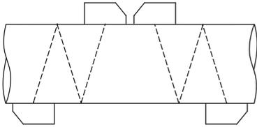
Fig. 3.5: Reflection arrangement with 1 beam and 4 sound paths
