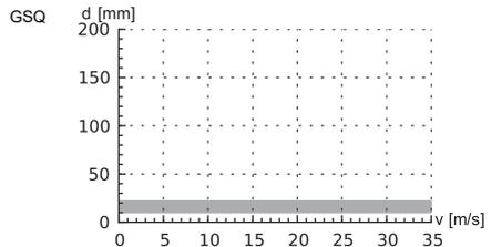
1 inner pipe diameter and max. flow velocity for a typical application with natural gas, nitrogen, oxygen in reflection arrangement with 2 sound paths (Lamb wave transducers)/1 sound path (shear wave transducers)
