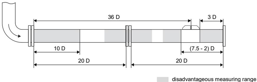
Considering flow profile and influence of noise, the measuring point can be selected in the area  $3 \dots (7.5 - 2) D$  on the right side of pipe segment 2 (with max. distance from the elbow).
