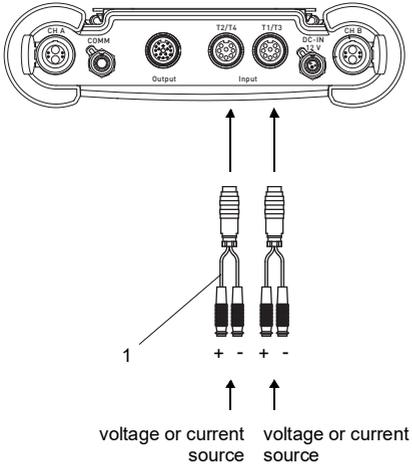
1 – adapter for voltage and current inputs
