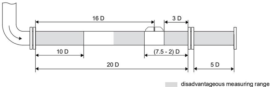
In the example, there is no area where both demands are met at the same time. The measuring point has to be selected as far as possible from the elbow, at a point where the influence of noise can be neglected:  $3 \dots (7.5 - 2) D$  on the right side of pipe segment 1. In the example, a distance of  $16 D$  from the elbow was selected.
