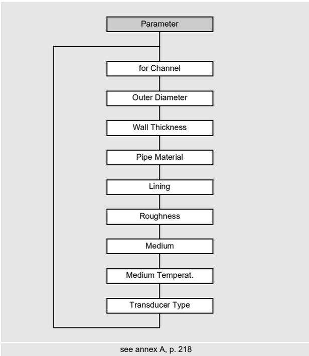
The pipe and fluid parameters are entered for the selected measuring point. The parameter ranges are limited by the technical characteristics of the transducers and the transmitter.
