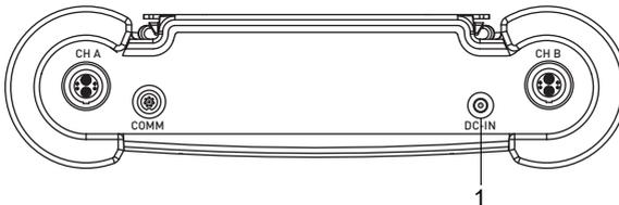
1 – power supply unit/battery charging unit
