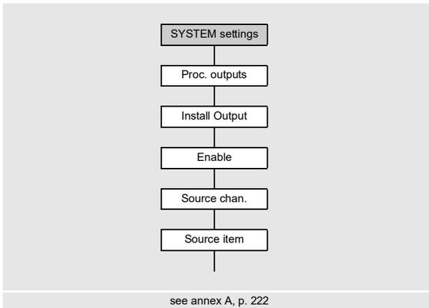
If the transmitter is equipped with outputs, they have to be installed and activated before they can be used:
