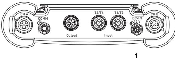
1 – power supply unit/battery charging unit
