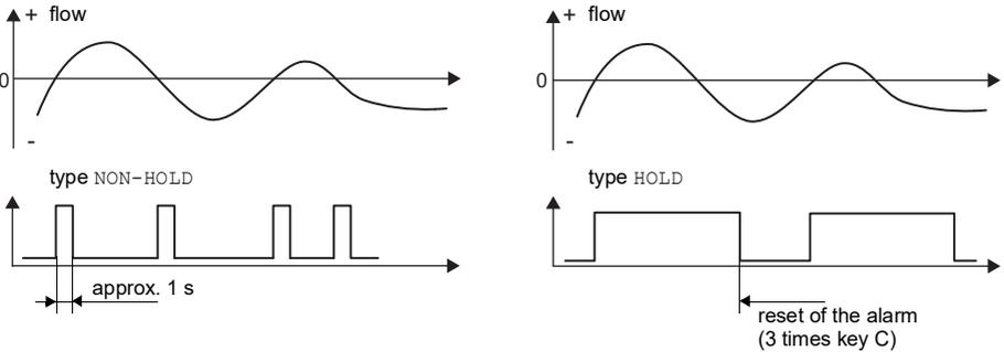
When adjusting to changed measurement conditions e.g. a substantial increase of the fluid temperature, the alarm will not be switched. Alarm outputs with the switching condition OFF will be set automatically to the switching function NO Cont.
