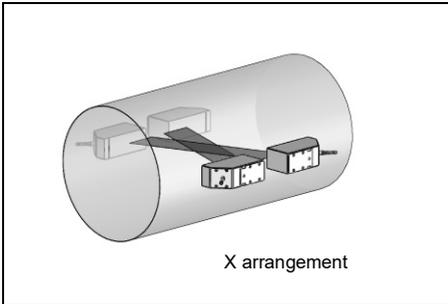
**Reflection arrangement with 2 beams and 2 planes**
