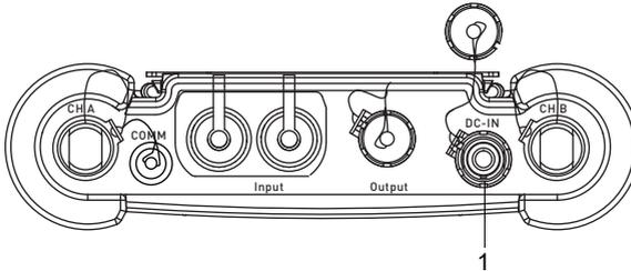
1 – power supply unit/battery charging unit
