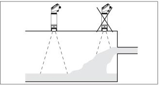
Fig. 5: Mounting of the radar sensor with inflowing medium
