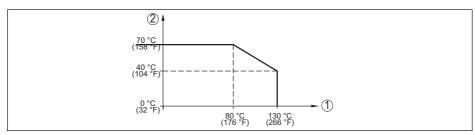
Fig. 19: Temperature derating VEGAPULS 42
