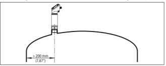
Fig. 3: Mounting of the radar sensor on round vessel tops
