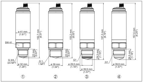
Fig. 20: Dimensions VEGAPULS 42 without display
