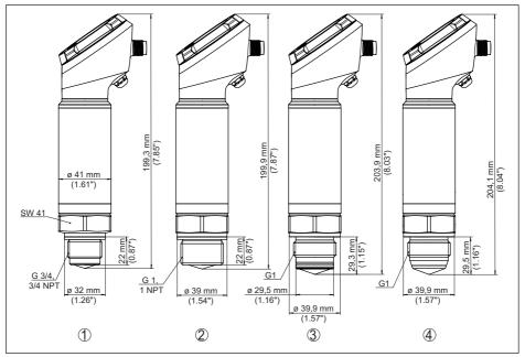
Fig. 21: Dimensions VEGAPULS 42 with display
