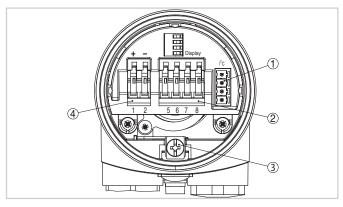
Electronics and terminal compartment, single chamber housing
