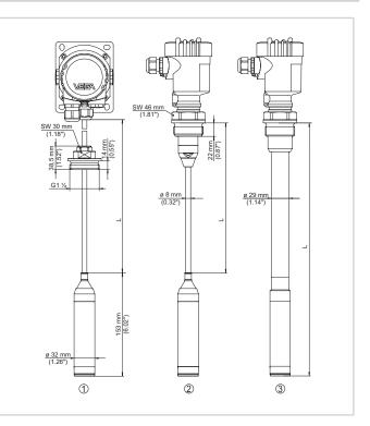
1 Version with suspension cable and threaded fitting unassembled G11/2
