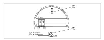
Electronics and terminal compartment, single chamber housing
