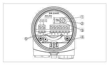
Electronics and connection compartment, single chamber housing
