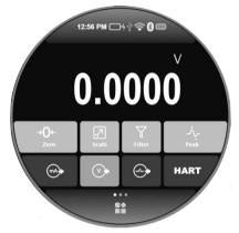
Figure 6 Electrical signal measurement function
