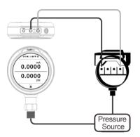
Figure 13 Calibrate pressure transmitter
