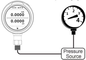
Figure 12 Calibrate Dial Pressure Gauge
