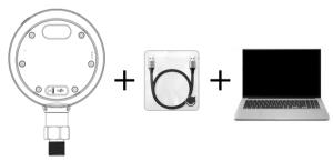
Figure 21 Connect to PC through the adapter
