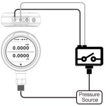
Figure14 Calibrate Pressure Switch
