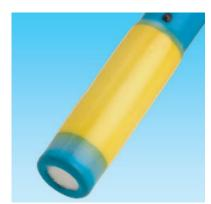
The reference electrode is integrated in the probe head, separately from the measuring electrode. The electrolyte connection between the electrolyte vessel, the reference electrode and the product to be measured is made using a tube and quick-action coupling and a shrunk, aseptic ground diaphragm.
