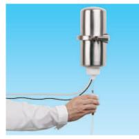
The pH Reiner probe is installed directly in a reactor nozzle or in the main current of a pipe. It may remain in the process zone all the time - even if the reactor is empty. The probe can be installed in any orientation and may remain dry without any limitations.
