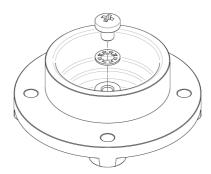
The use of the internal earth connection as the only earthing connection may be acceptable with wiring systems using steel wire armoured cable or metallic conduit. For all other installations an external earthing connection must be used which may be connected to the external threaded mounting holes on the flowmeter body or using metallic cable glands with earthing tags.
