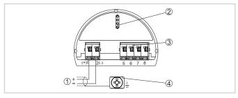
Secondary terminal connections (intrinsically safe devices)
