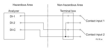
Figure 5.7 Contact Input Wiring
