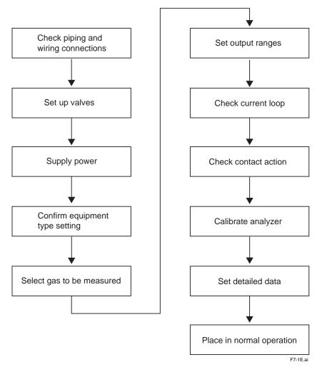
Figure 7.1 Startup Procedure
