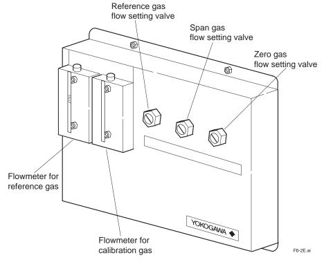
Figure 6.2 ZA8F Flow Setting Unit
