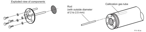
Figure 11.1 Cleaning the Calibration Gas Tube
