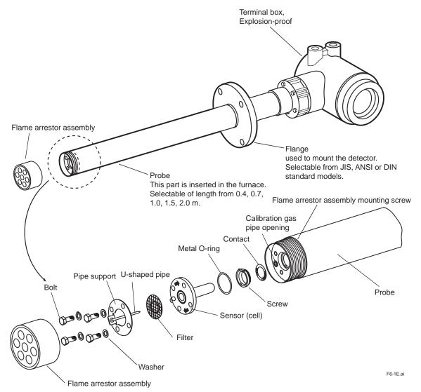
Figure 6.1 Integrated type Explosion-proof Zirconia Oxygen Analyzer
