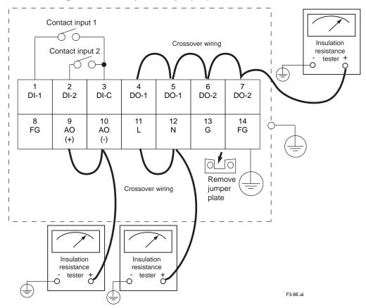
Figure 3.10 Insulation Resistance Test
