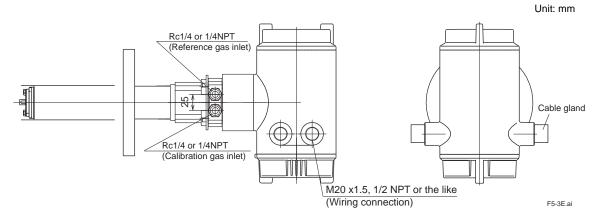
Figure 5.3 Cable Gland Mounting
