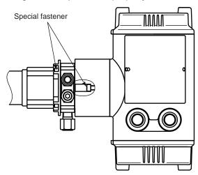
Figure 3.4 Special fastener
