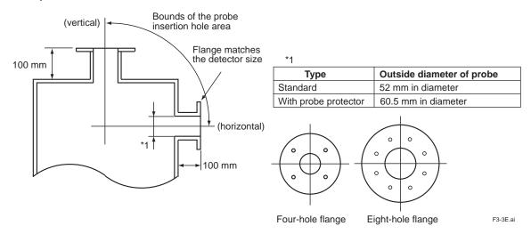
Figure 3.5 Example of forming probe insertion hole
