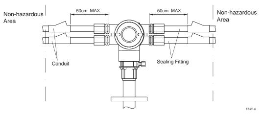
Figure 3.3 Wiring of ZR202S-C
