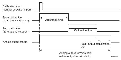
Figure 9.4 Calibration and Hold (Output stabilization) Time Settings
