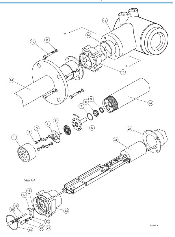
Figure 11.4 Exploded View of Detector
