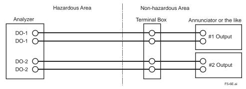
Figure 5.6 Contact Output Wiring
