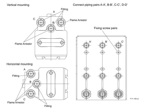
Figure 11.10 Fixing Flowmeter
