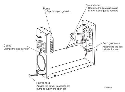
Figure 10.4 Standard Gas Unit Component Identification
