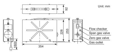
Zero gas cylinder (6 cylinder): E7050BA
