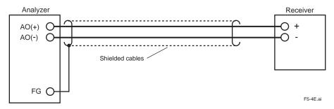
Figure 5.4 Wiring for Analog Output
