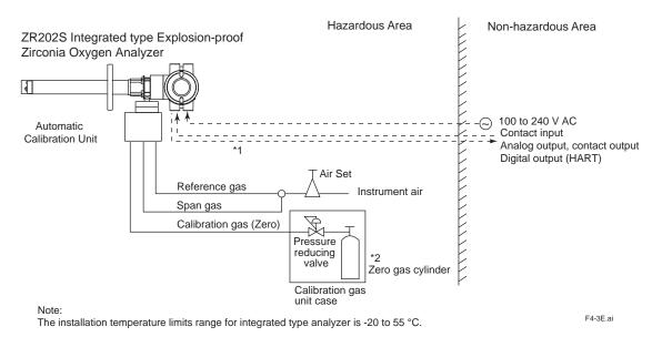
Figure 4.3 Piping for System 2
