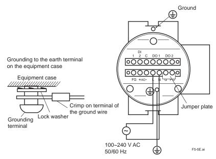
Figure 5.5 Power and Grounding Wiring
