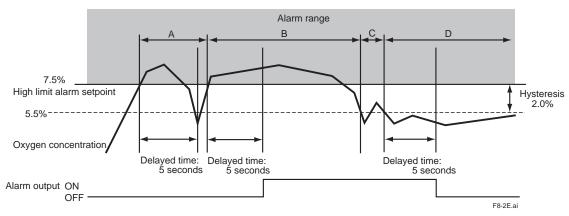
Figure 8.2 Alarm Output Action
