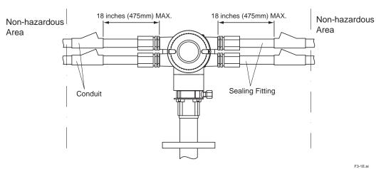
Figure 3.2 Wiring of ZR202S-B
