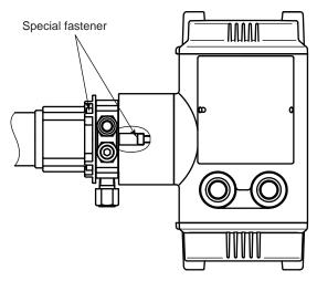
Figure 3.1 Special fastener
