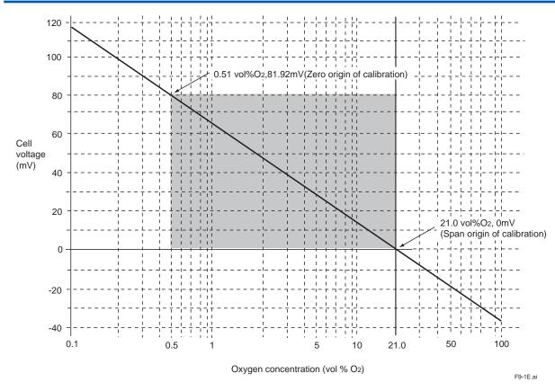
Figure 9.1 Oxygen Concentration in a Measurement Gas vs. Cell Voltage (21 vol%O<sub>2</sub> Equivalent)
