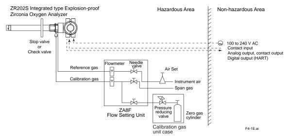
Figure 4.1 Piping for System 1
