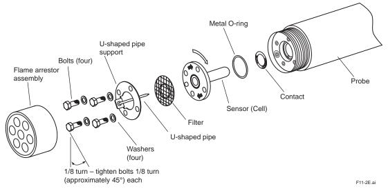
Figure 11.2 Exploded View of Sensor Assembly
