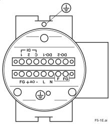
Figure 5.1 Terminals for External Wiring
