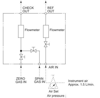
Air pressure ; without check valve ; sample gas pressure + approx.50 kPaG
