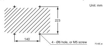
Figure 3.8 Mounting holes
