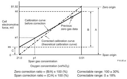
Figure 10.2 Span gas and Zero gas Correction Ratios
