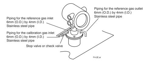
Figure 4.2 Piping for the Calibration Gas Inlet
