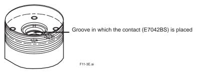
Figure 11.3 Installing the Contact
