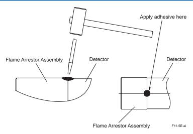
Figure 11.5 Removal of Flame Arrestor
