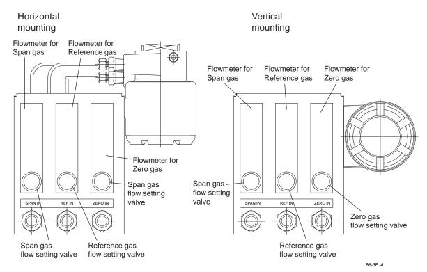
Figure 6.3 Automatic Calibration Unit
