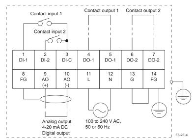
The protective grounding for the analyzer shall be connected either the protective ground terminal in the equipment or the ground terminal on the case. Standard regarding grounding: Ground to earth, ground resistance:  $100 \Omega$  or less.
