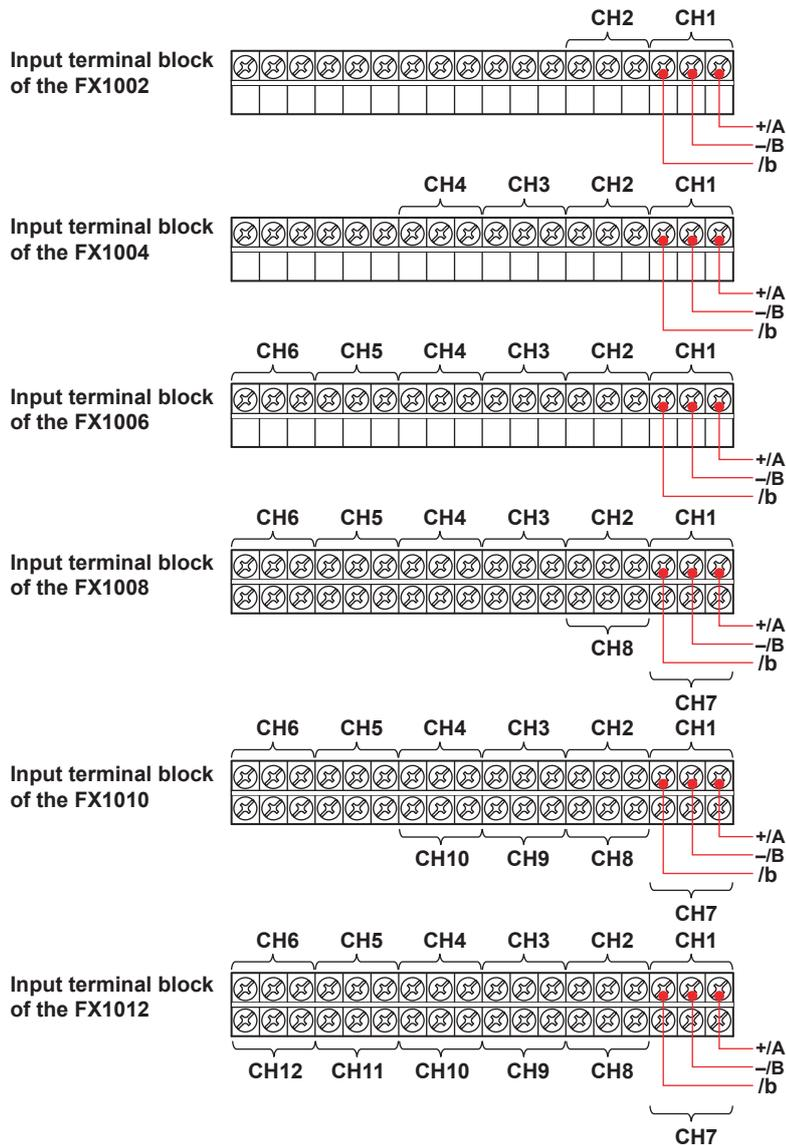
For TC input, use shielded compensating lead wires for wiring.
