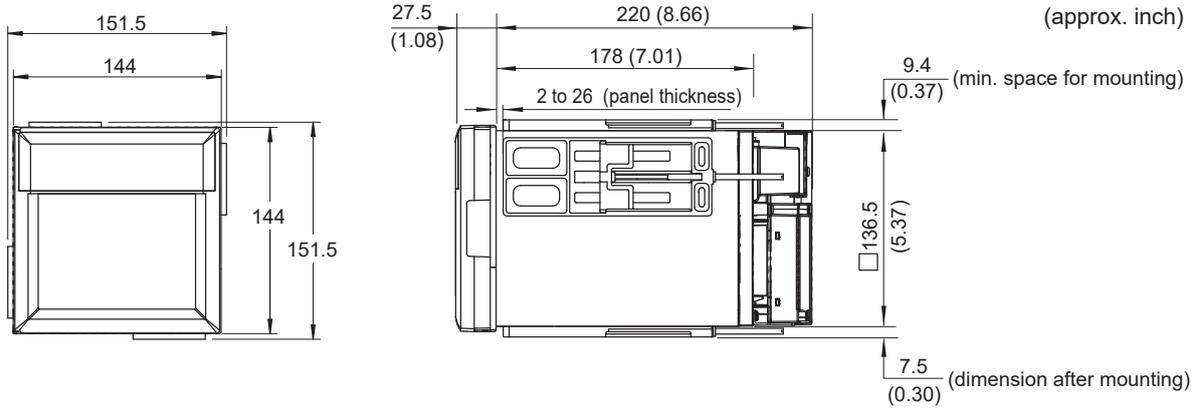
Note: The  $\mu$ R10000 should be mounted by only two brackets, either on the top & bottom of the recorder, or on the left & right side of the recorder.
