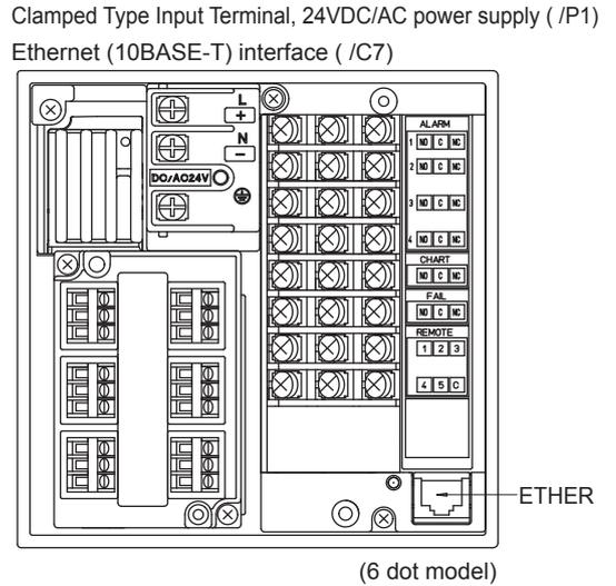
If /C7 is specified and /A□ and /R1 are not specified, the function of the accessory screw terminal block is not available.
