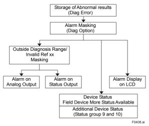
Figure 4.6 Alarm and Alert Setting
