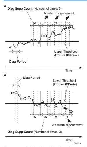
Figure 4.4 Relationship of Diag Supp Count and Alarm
