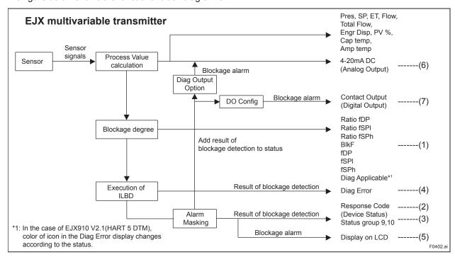
Figure 4.2 Functional Block Diagram of ILBD
