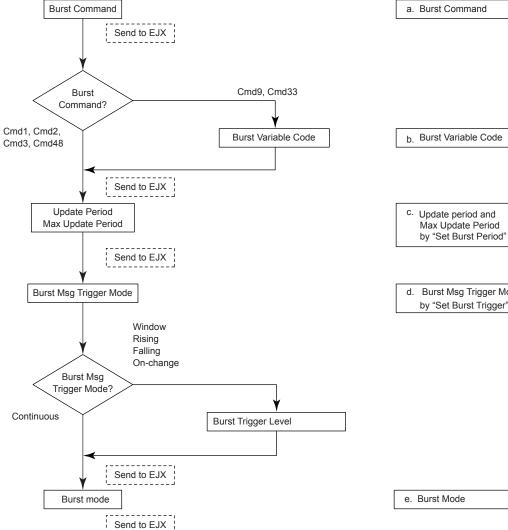
d. Burst Msg Trigger Mode by "Set Burst Trigger"
