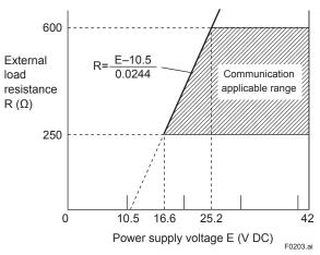
Figure 2.3 Relationship between Power Supply Voltage and External Load Resistance
