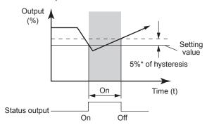
\*: 5% of setting span for differential pressure / pressure
