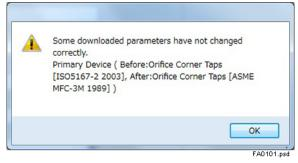
The calibration of the transmitter must be performed after parameters are set.
