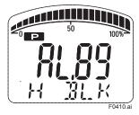
Figure 4.7 Display Example of H Side Blocking
