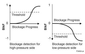
Figure 4.3 Relation between Blockage Progress and BlkF
