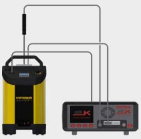
Our ADVANCED blocks include built in automatic temperature cycling with the ability to program with up to 25 set temperatures. Temperature ramp and hold cycles can also be created. Up to 100 separate programs can be stored and all data is automatically logged.
