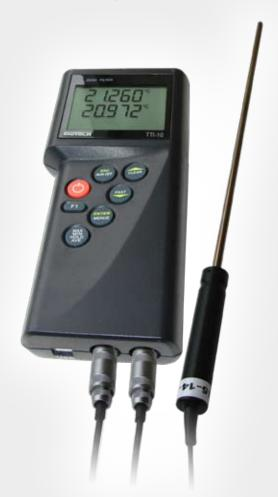
The TTI-10 brings laboratory level performance of up to 0.01°C (10mK) and resolution up to 0.001°C (1mK) in a portable handheld instrument. Battery life is typically 20 hours from a 9V PP3 alkaline battery and a protective rubber boot, that is included as standard, offers protection in field use.
