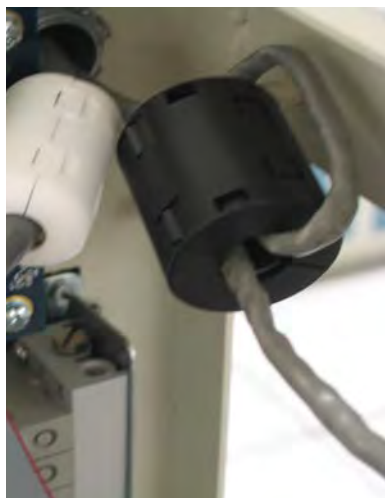
Figure 13: Ethernet Cable Passing through Ferrite
