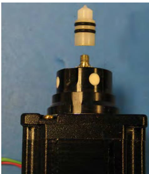
Figure 100: The High Pressure Valve Seal — After Removal
