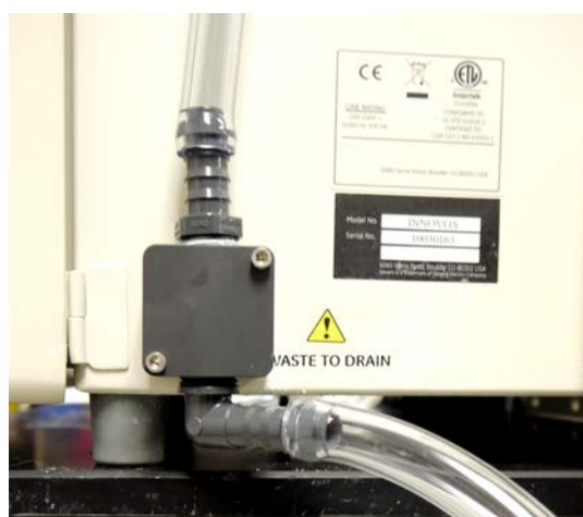
Figure 5: Connecting the Waste Lines on the Waste Block
