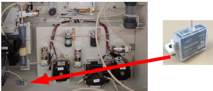
Figure 83: Liquid Sensor Location — Analyzer Enclosure
