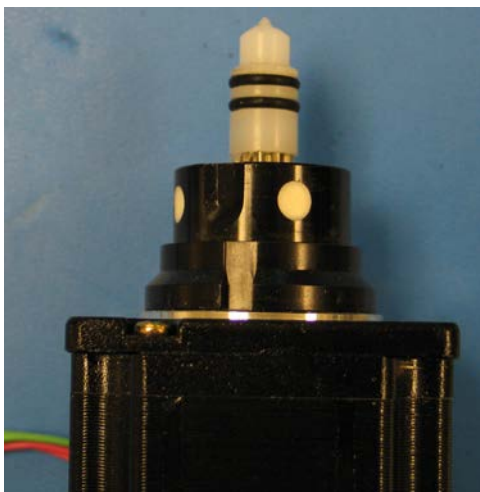
Figure 99: The High Pressure Valve Seal — Before Removal
