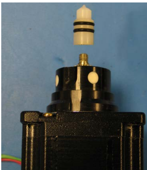
Figure 100: The High Pressure Valve Seal — After Removal
