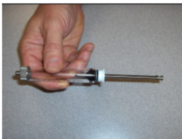
Figure 94: Pulling Out the Plunger
