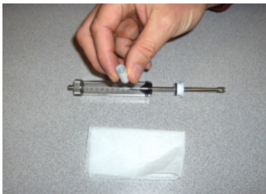
Figure 95: Removing the Stopper
