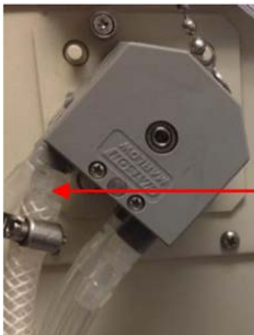
Figure 28: Overflow Mode — 2-Stream, External Sample Peristaltic Pump Position
