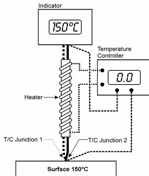
Figure 4. Automatic Thermally Compensated Probe With Control & Indication.
