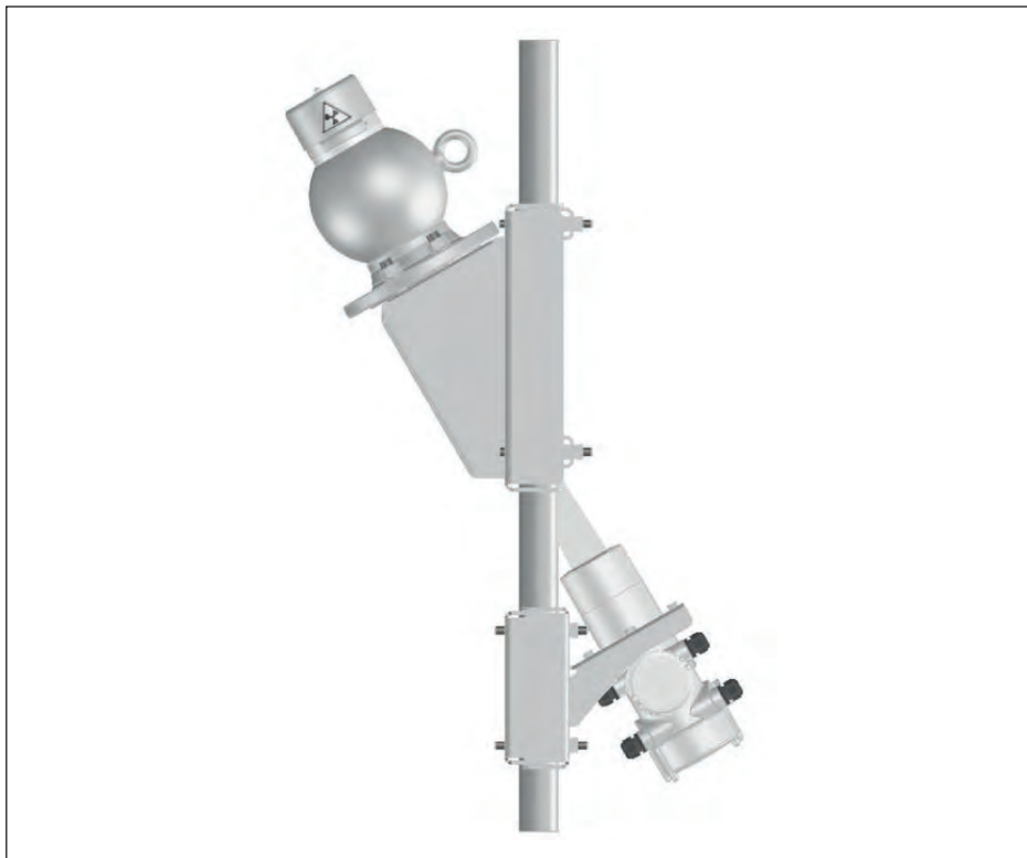
Fig. 56: Mounting brackets for diagonal mounting on pipes from 50 ... 220 mm (1.97 ... 8.66 in)
