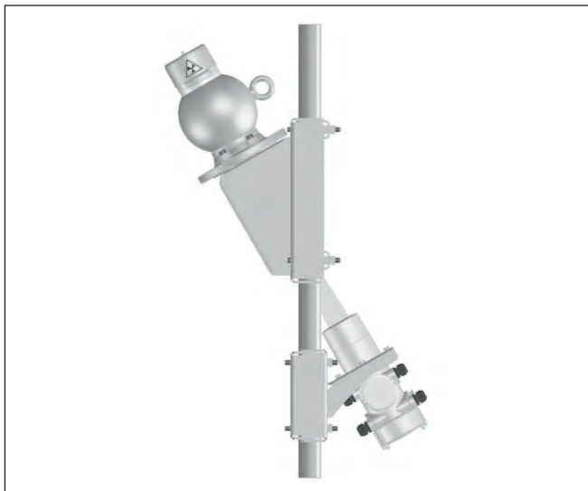
Fig. 18: 30° measurement setup on a pipeline with diameter 50 ... 100 mm (1.97 ... 3.94 in)
