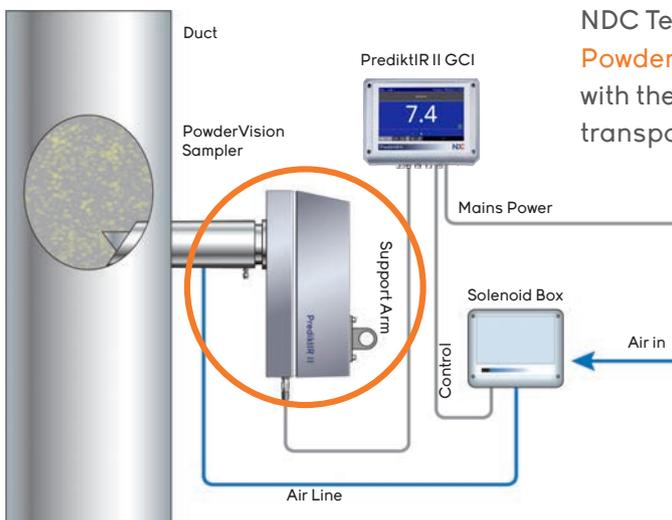
NDC Technologies' pneumatic PowderVision sampler can be used with the PrediktIR II gauge for powders transported in enclosed ducts.
