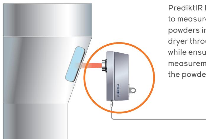
PrediktIR II can be installed to measure moisture in powders in a fluid bed dryer through a sight glass, while ensuring that the measurement area is below the powder line.
