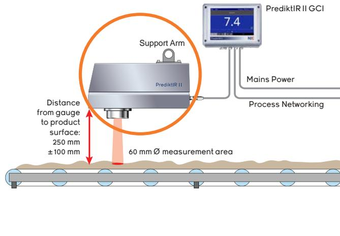
PrediktIR II measures over a 60 mm diameter standard beam patch size. It is suspended over the process line at a distance of 250 mm from the mean product height and tolerates product height fluctuations of  $\pm 100$  mm.
