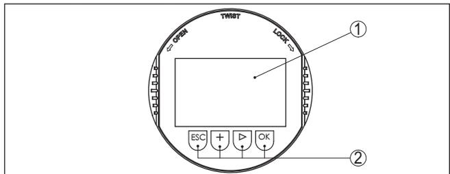
Fig. 38: Display and adjustment elements
