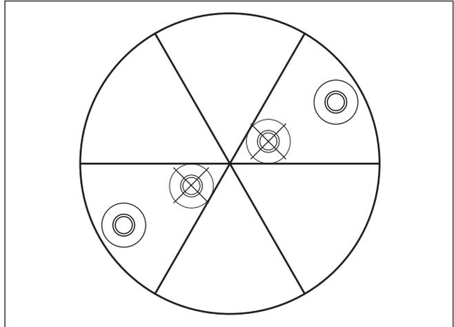
Fig. 21: Mounting of VEGAPULS SR 68 in multiple chamber silos
