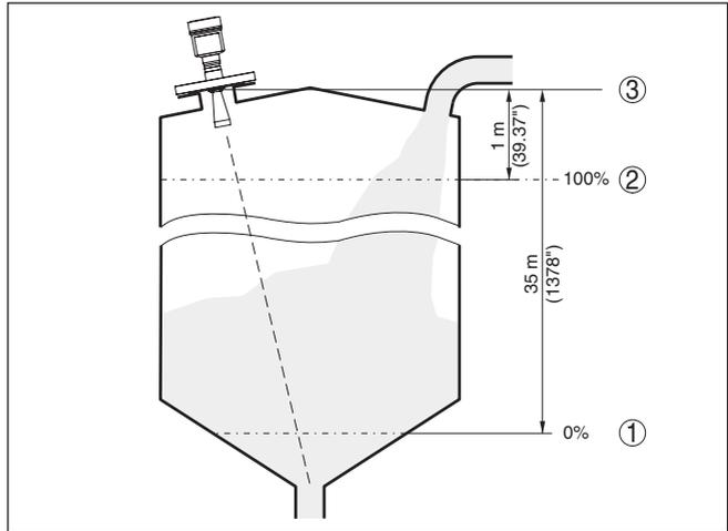
Fig. 40: Parameterisation example, Min./max. adjustment
