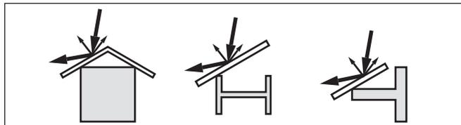
Fig. 16: Cover flat, large-area profiles with deflectors
