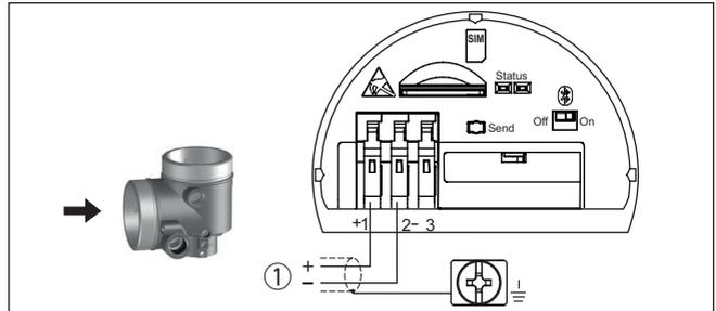
Fig. 29: Connection compartment - Radio module PLICSMOBILE 81
