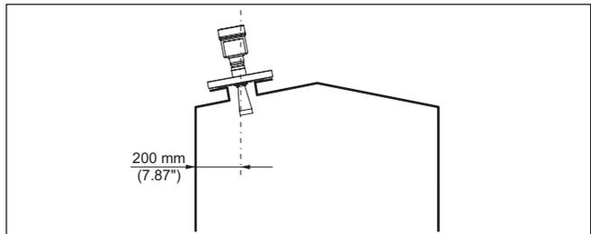
Fig. 5: Mounting the radar sensor on the vessel top
