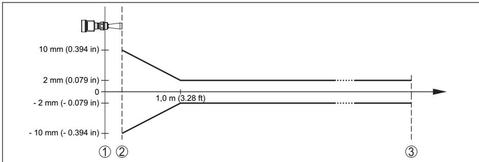
Fig. 55: Deviation under reference conditions
