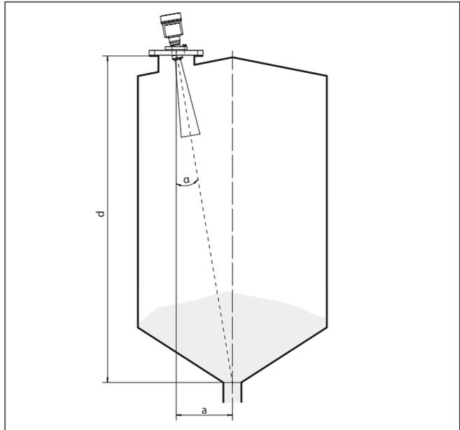
Fig. 14: Proposal for installation after orientation VEGAPULS SR 68
