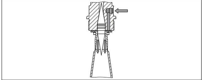
Fig. 23: Purging air connection with horn antenna
