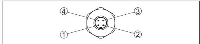
Fig. 34: View to the plug connector M12 x 1
