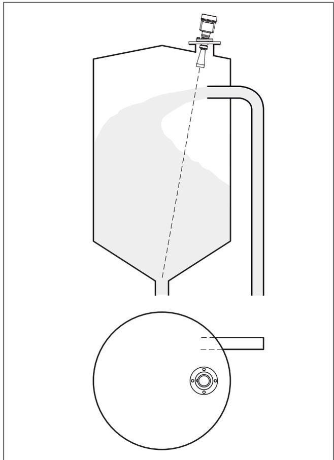
Fig. 7: Mounting of the radar sensor with inflowing medium
