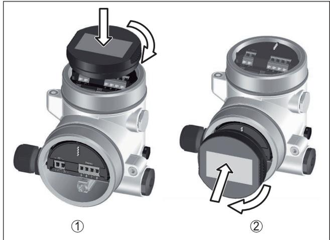
Fig. 37: Installing the display and adjustment module in the double chamber housing
