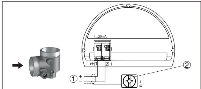
Fig. 31: Connection compartment - Ex-d-ia double chamber housing
