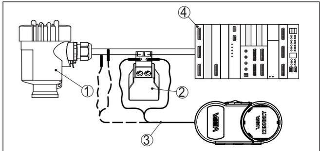
Fig. 42: Connecting the PC via HART to the signal cable
