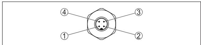
Fig. 32: Top view of the plug connector
