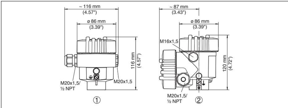
Fig. 57: Housing versions with protection rating IP 66/IP 68 (0.2 bar) (with integrated display and adjustment module the housing is 18 mm/0.71 in higher)
