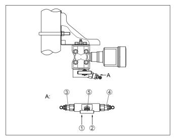
Fig. 10: Connection of a 3-fold valve block
