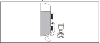
Fig. 5: Density measurement with VEGADIF 85
