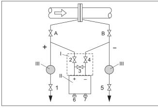
Fig. 39: Preferred measurement setup for liquids
