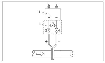
Fig. 38: Prefered measurement setup for gases, connection via 3-fold valve block, flanging on both sides
