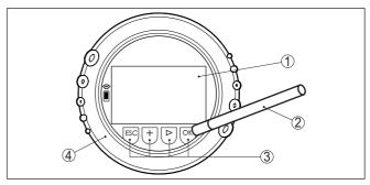
Fig. 34: Display and adjustment elements - with adjustment via magnetic pen
