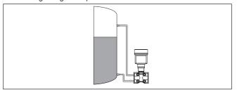
Fig. 2: Level measurement with VEGADIF 85 in a pressurized vessel
