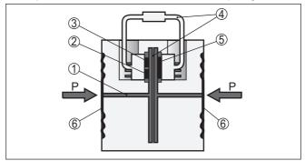
Fig. 7: Configuration metallic measuring cell
