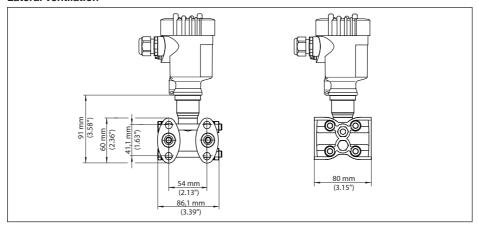
Fig. 47: VEGADIF 85, 1/4-18 NPT connection, with lateral ventilation
