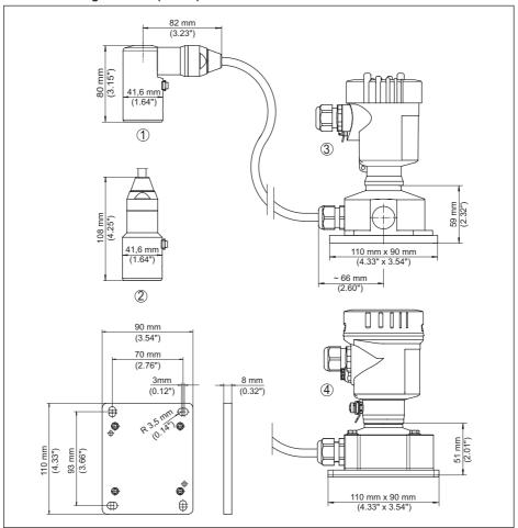
Fig. 45: IP68 version with external housing
