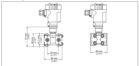
Fig. 46: VEGADIF 85, ventilation on process axis
