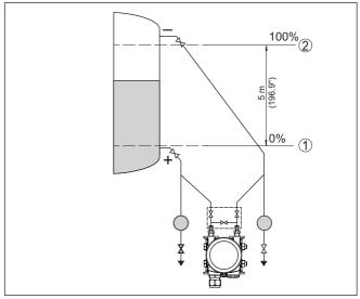
Fig. 35: Parameter adjustment example "Min./max. adjustment, level measurement"
