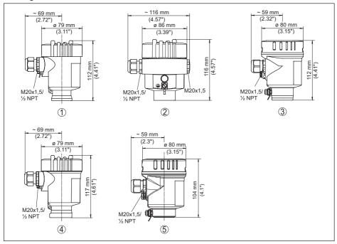
Fig. 44: Housing versions with protection rating IP66/67 and IP66/IP68 (0.2 bar) - with integrated display and adjustment module the housing is 9 mm/0.35 in higher, with Aluminium and stainless steel precision casting housings 18 mm/0.71 in
