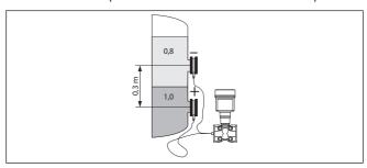
Fig. 25: Measurement setup with interface measurement
