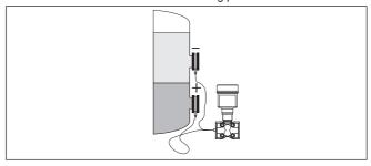
Fig. 6: Interface measurement with VEGADIF 85
