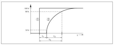
Fig. 42: Behaviour in case of sudden change of the process variable.  $t_i$ : dead time;  $t_{2}$ : rise time;  $t_{3}$ : jump response time
