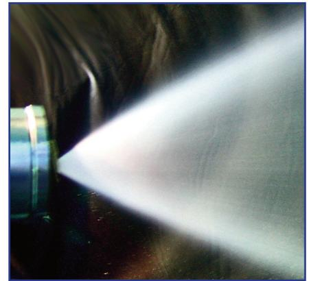
To approach VARIfix vortex type nozzles a look to the plain area devices is necessary with particular regards to the rangeability characteristic. Fixed area plain nozzles have a constant flow rate changes.
