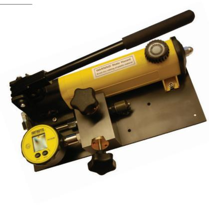
High accuracy and stability - is achieved by use of a piezoresistive transducer with a built-in temperature compensation. Unlike some other pressure calibrators, accuracy is maintained when decreasing pressure which makes the unit ideal for verification of hysteresis. All units are calibrated in positive as well as in negative direction.
