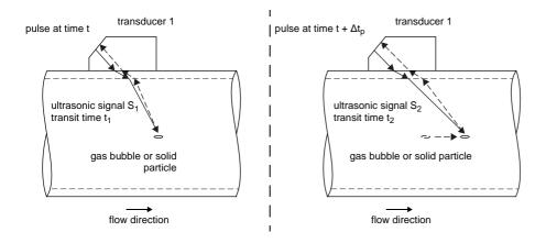
The average flow velocity of the fluid is calculated as follows:
