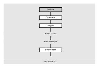
If the transmitter is equipped with outputs, they have to be configured. For the configuration of the analog output, see section 9.2.6.
