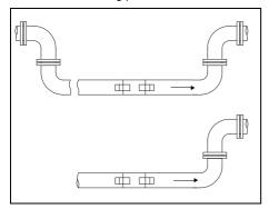
Fig. 3.15: Disadvantageous transducer mounting position
