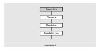
The measuring channels to be used for calculation and the calculation function have to be entered in the program branch Parameters.
