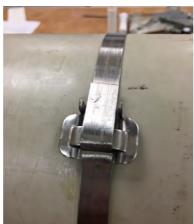
• Fold the tabs of the clip over the solid band and cut the protruding band off (see Fig. 6.76).
