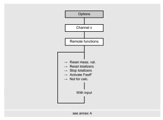
Remote functions can be triggered by event triggers, triggerable analog inputs or binary inputs.
