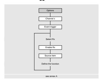
It is possible to configure max. 4 independent event triggers per channel: R1, R2, R3 and R4.
