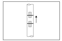
Fig. 3.13: Disadvantageous transducer mounting position
