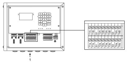
1 - connection of the temperature probe
