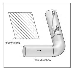
The sound beam plane is selected at an angle of 90° ± 45° to the elbow plane.
