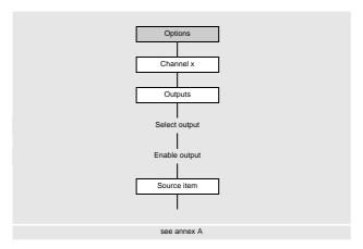
If the transmitter is equipped with outputs, they have to be configured. The measured value, the status value or an event value can be transmitted via the different outputs. In the following, the configuration of an analog output is described.
