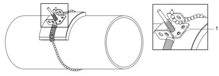
1 - slots on the upper side of the temperature probe
