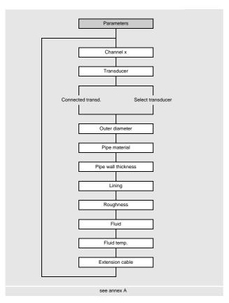
The pipe and fluid parameters are entered for the selected measuring point. The parameter ranges are limited by the technical characteristics of the transducers and the transmitter.
