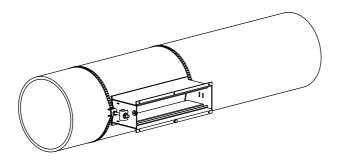
Fig. 6.64: Tension strap through rail fixture
