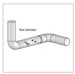
The sound beam plane is selected according to the nearest elbow (horizontal or vertical, depending on the pipe orientation, see above).
