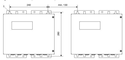
1 - fixing hole for wall mounting Ø 9.5
