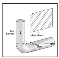
The sound beam plan is selected at an angle of 90° to the elbow plane. The elbow is upstream of the measuring point.
