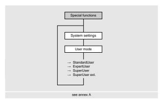
The user modes allow extended diagnostics of signals and measured values as well as the definition of additional parameters adapted to the application.
