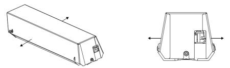
Fig. 6.37: Disassembly of the transducer mounting fixture Variofix C
