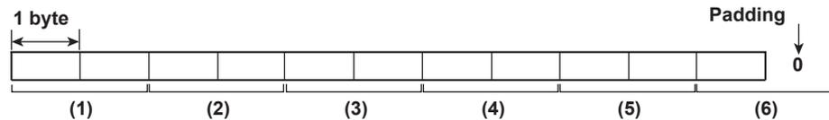
If the data length of the buffer is odd, a zero is padded so that it is even. (1) through (6) are summed as unsigned two-byte integers (unsigned short). If the digit overflows a 1 is added. Finally, the result is bit-wise inverted.
