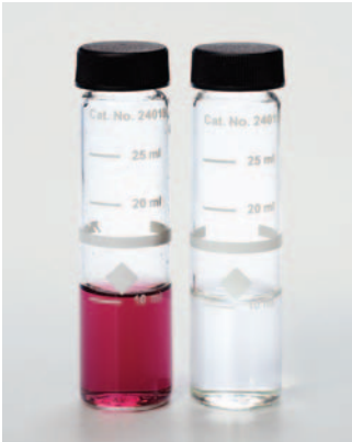
Measuring free available chlorine levels in water using a manual colorimeter. The pink "in" beaker shows flow stream in which chlorine is detected. The clear "out" beaker shows water after treatment with PharmaGuard – no chlorine detected.
