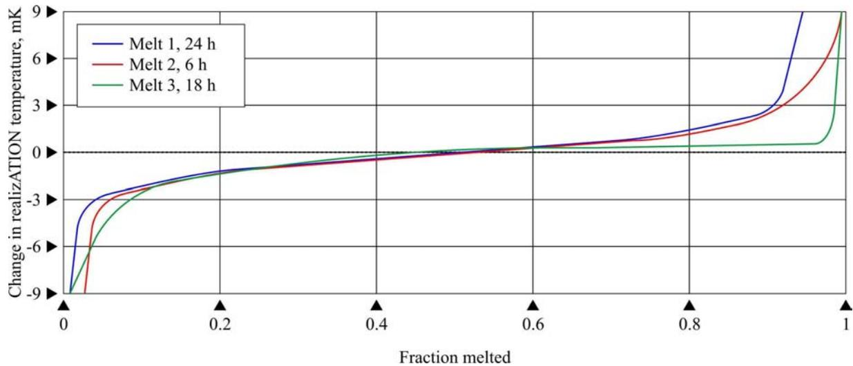
Graph 2. Freezing curves for the Isotech Al fixed point cell (Isotech model ITL-M-17672-O, Serial No. Al 188)
