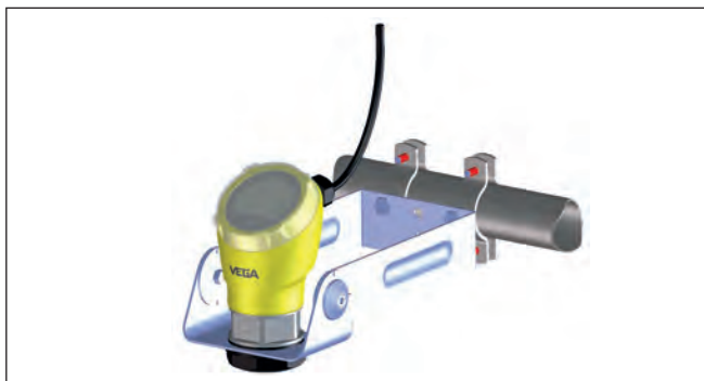
Fig. 15: Mounting bracket for pipe mounting horizontally over pipe clamps provided by customer
