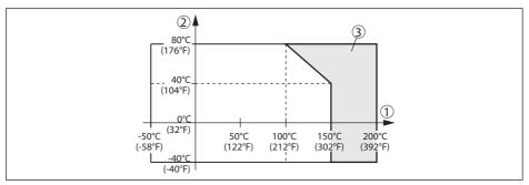
Fig. 31: Ambient temperature - Process temperature
