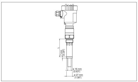
Fig. 39: VEGACAL 65, screening tube, for example against strong condensation
