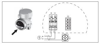
Fig. 15: Wiring plan - double chamber housing
