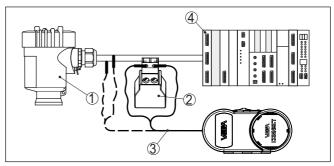
Fig. 25: Connecting the PC via HART to the signal cable
