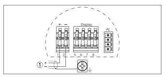
Fig. 11: Wiring plan - single chamber housing
