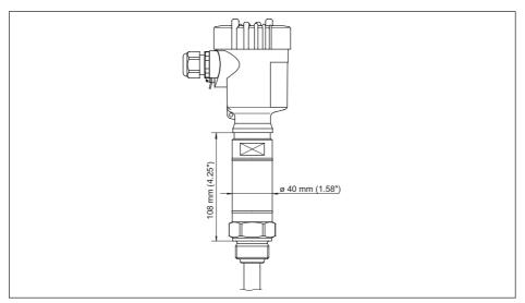
Fig. 38: Temperature adapter
