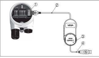
Fig. 24: Connection via interface adapter VEGACONNECT external
