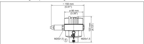
Fig. 34: Housing version with protection rating IP66/IP68 (1 bar), (with integrated display and adjustment module the housing is 18 mm/0.71 in higher)
