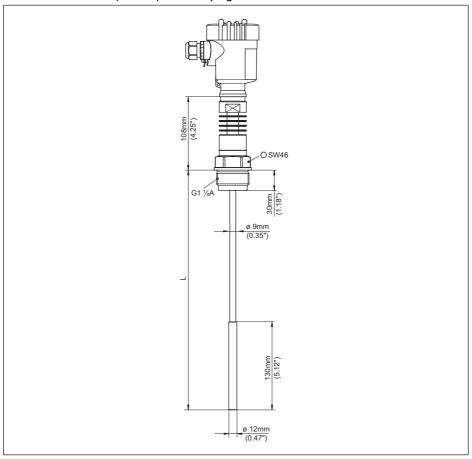
Fig. 37: VEGACAL 65, PTFE-insulated cable (ø 8 mm) with crimping sleeve / -50 ... +200  $^{\circ}\text{C}$
