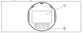
Fig. 22: Display and adjustment elements
