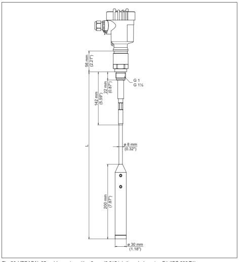
Fig. 36: VEGACAL 65, cable version with ø 8 mm (0.315 in), threaded version G1 (ISO 228 T1)
