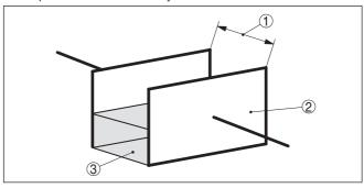
Fig. 3: Functional principle - Plate capacitor
