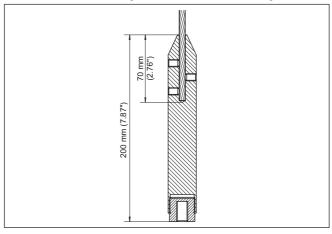
Fig. 30: Take the gravity weight into account and shorten the cable respectively
