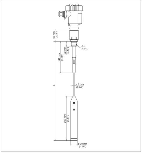
Fig. 35: VEGACAL 65, cable version with ø 6 mm (0.236 in), threaded version G1 (ISO 228 T1)
