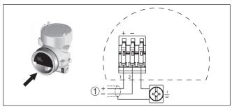
Fig. 19: Wiring plan, Ex-d-ia double chamber housing
