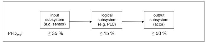
Fig. 2 usual fraction of PFD<sub>avg</sub> to the subsystems
