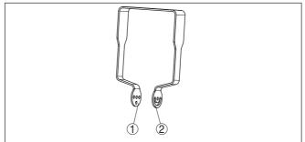
Fig. 8: Mounting strap for screwing to the sensor
