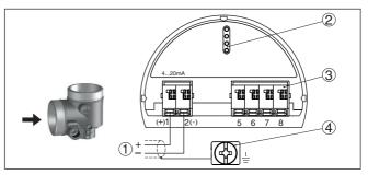
Fig. 39: Connection compartment - double chamber housing
