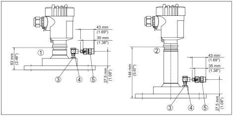
Fig. 65: VEGAPULS 69, metal-jacketed lens antenna with rinsing connection
