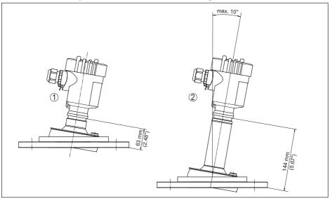
Fig. 66: VEGAPULS 69, metal-jacketed lens antenna and swivelling holder
