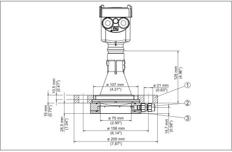
Fig. 69: VEGAPULS 69 with compression flange suitable for flanges 3" 150 lbs, DN 80 PN 16 and rinsing connection
