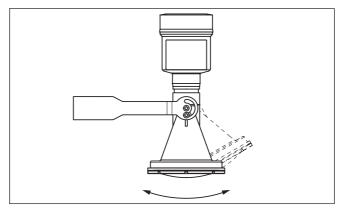
Fig. 9: Adjustment of the angle of inclination
