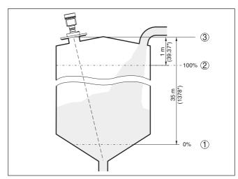
Fig. 47: Parameterisation example, Min./max. adjustment
