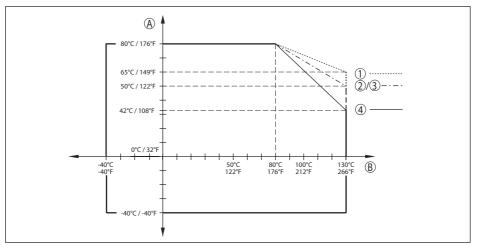
Fig. 57: Derating, ambient temperature, thread G11/2 with integrated horn antenna up to +130 °C (+266 °F)
