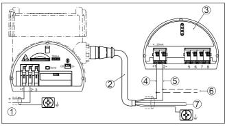
Fig. 37: Connection voltage supply and plics® sensor
