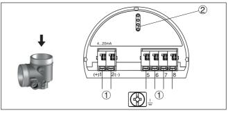
Fig. 38: Electronics compartment - Ex-d double chamber housing
