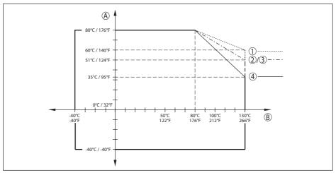
Fig. 54: Derating, ambient temperature, metal-jacketed lens antenna up to +130 °C (+266 °F)
