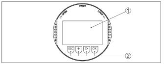
Fig. 45: Display and adjustment elements
