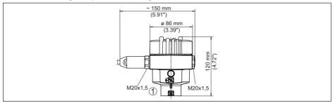
Fig. 61: Housing version with protection rating IP66/IP68 (1 bar), (with integrated display and adjustment module the housing is 18 mm/0.71 in higher)
