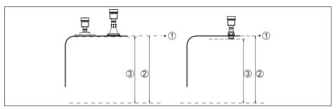
Fig. 52: Data of the input variable, on the left flange with lens antenna and plastic horn antenna, on the right thread with integrated horn antenna
