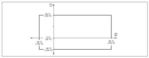
Fig. 56: Derating, ambient temperature, plastic horn antenna
