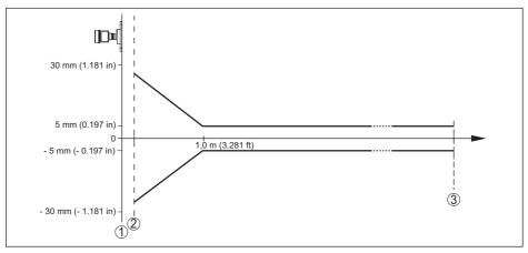
Fig. 53: Deviation under reference conditions
