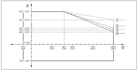
Fig. 58: Derating, ambient temperature, thread G11/2 with integrated horn antenna up to +200 °C (+392 °F)
