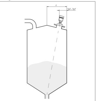
Fig. 18: Mounting position and orientation
