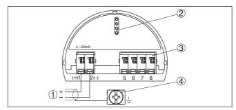
Fig. 30: Electronics and connection compartment - single chamber housing
