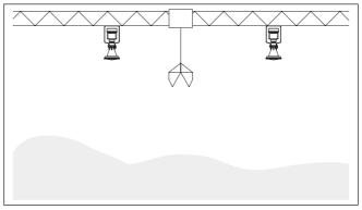
Fig. 22: Radar sensors on traverse crane
