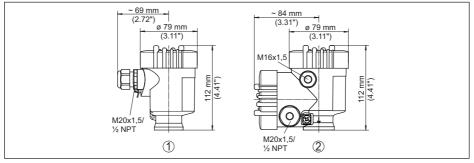
Fig. 59: Housing versions in protection IP66/IP67 (with integrated display and adjustment module the housing is 9 mm/0.35 in higher)
