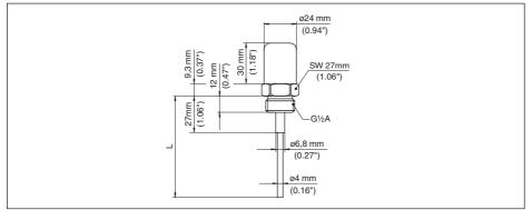
Fig. 5: Conductive rod electrode EL 8
